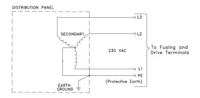
Figure 5: Earth Grounded WYE Distribution Transformer
